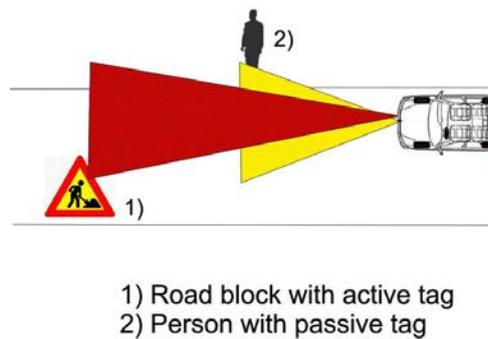
Figure 2. Combined use of passive and active tag with an harmonic radar
