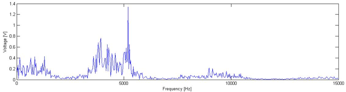
Figure 6: Spectra of the signals acquired from sensors without operating the control
