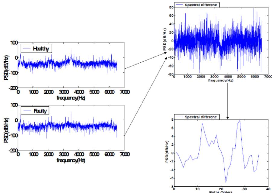
Figure 7. Procedure followed for obtaining the input data used for the fault detection technique
