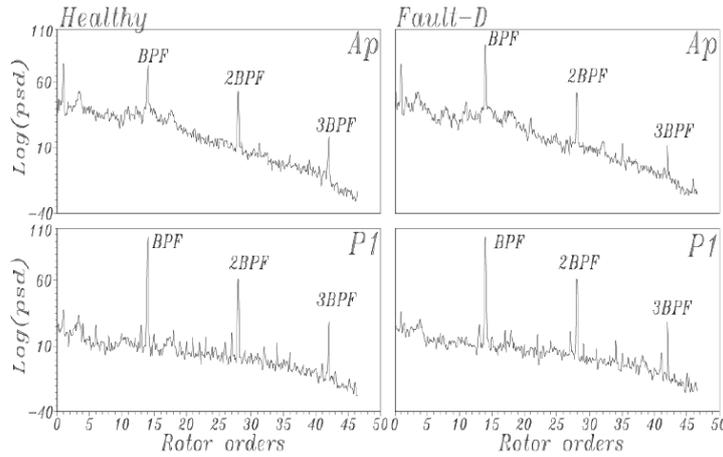
Figure 8. Acceleration (upper plots) and fluid pressure (lower plots) Power Spectral Density plots for healthy and faulty conditions
