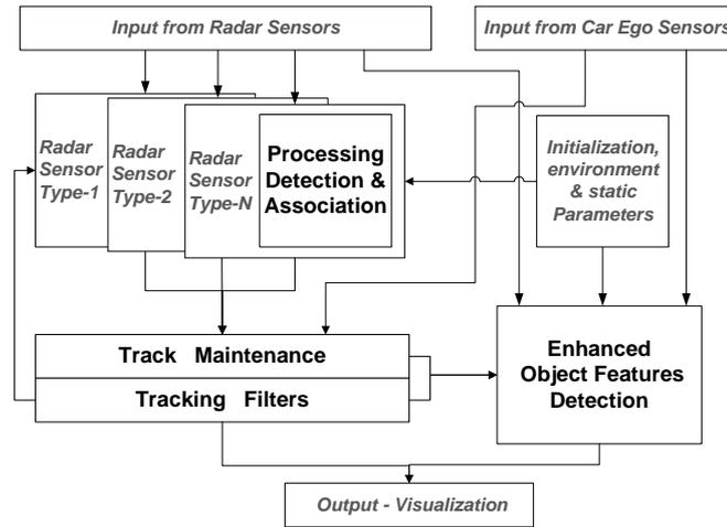
Figure 4. The Intelligent System for Enhanced Features Detection in the overall Radar ECU architecture.
