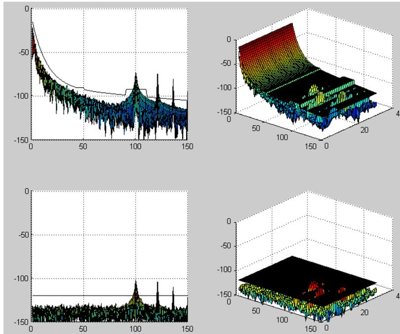
Figure 3. Simulated return signals from conventional (upper) & harmonic (lower) sensors
