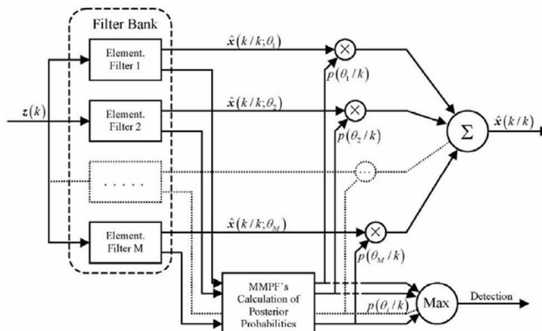
Figure 9. The general structure of the Multi-Model Partitioning Algorithm.
