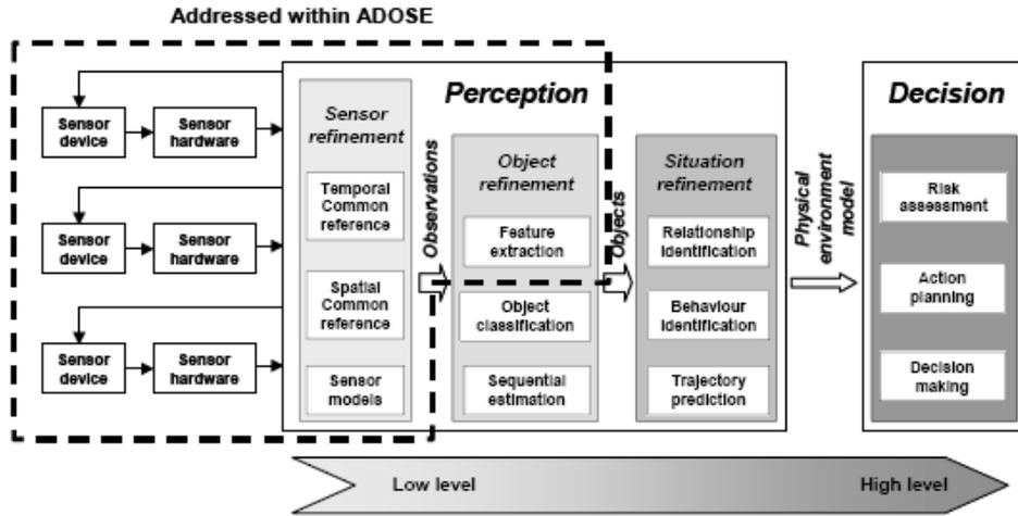
Figure 1. Data processing tasks of a typical driver assistance system and ADOSE objectives
