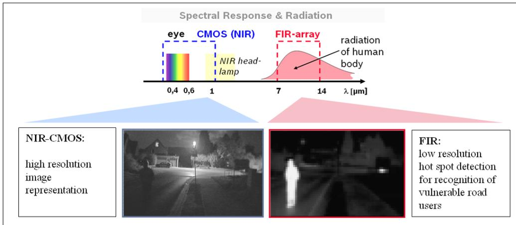
Fig. 1 Multi-spectral approach for warning night vision with NIR / FIR data fusion (top); identical night vision scene with different sensors (bottom): CMOS-NIR imager without active light (left) and low resolution FIR-array (right).
