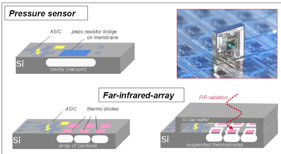
Fig. 2: From integrated pressure sensor to thermal imager. Top left: integrated pressure sensor principle; top right: picture of an integrated pressure sensor, the membrane is the square in the centre of the chip; bottom left: Instead of a single cavity for the pressure sensor an array of cavities is made (one beneath each pixel); bottom right: fully vacuum packaged thermal imager.
