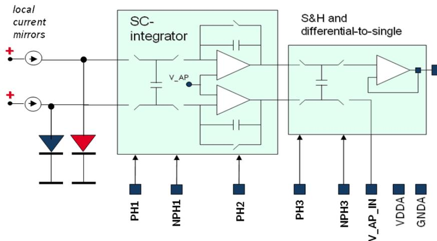
Fig. 4: Block diagram of SC integrator stage.
