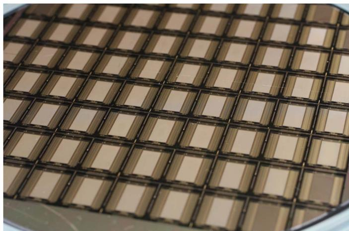
Fig. 3: Photograph of first ADOSE wafer
