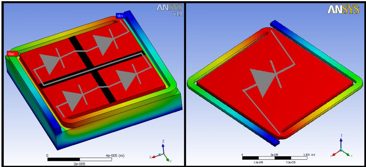
Fig. 4: Thermal simulation of a four-fold diode ADOSE pixel compared to the old single-diode design
