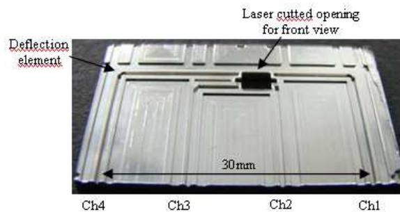
Fig. 3. Aluminum coated PMMA lightpipes with an opening for frontal vision function fabricated by laser cutting
