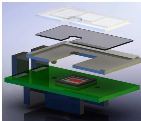
Fig. 4. Schematic of surface assembly of the lightpipes. From top to bottom: PMMA lightpipes, sealing foil, lightpipe holder with deflection element, CMOS imager mounted on PCB.
