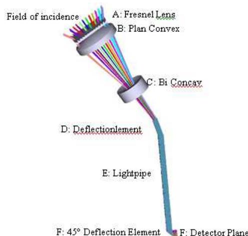
Fig. 2. Schematic diagram of the optical setup showing the optical components. The lightpipe is coated with a thin film of aluminum for enhanced reflection
