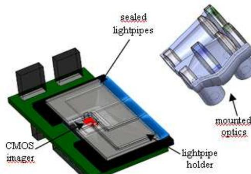
Fig.1. Schematic of the optical system
