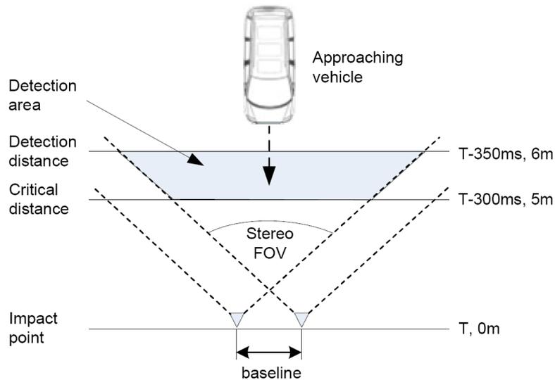
Figure 2. Stereo vision setup for the use in a pre-crash warning side impact detection application.
