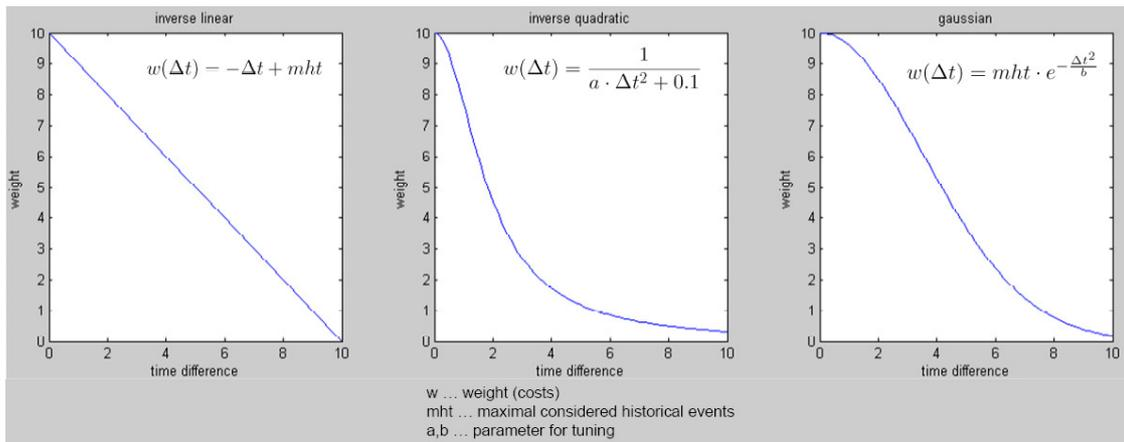
Figure 7. Weighting function for calculating the costs of matched address events.
