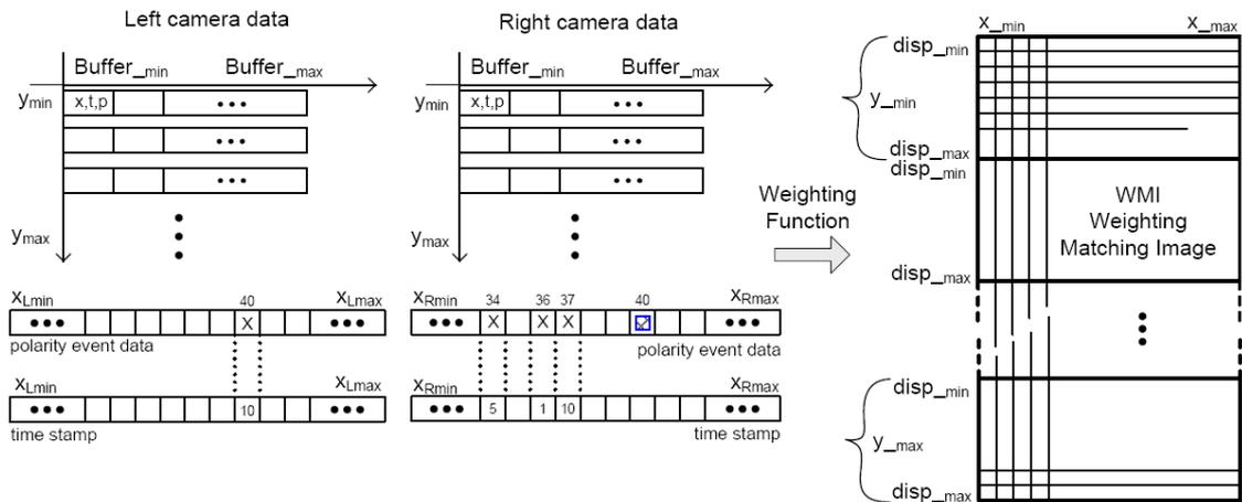
Figure 6. Matching and weighting of corresponding address events and writing of calculated costs into the WMI.
