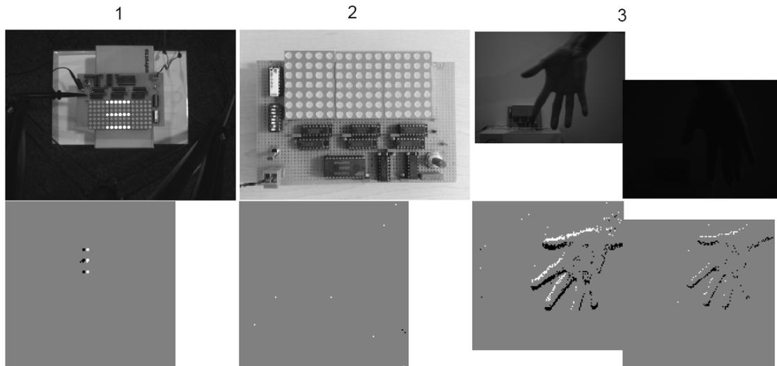
Figure 1. Comparison of a silicon retina sensor (second row) and a conventional camera (first row), (1) high temporal resolution, (2) data transmission efficiency, (3) high dynamic range
