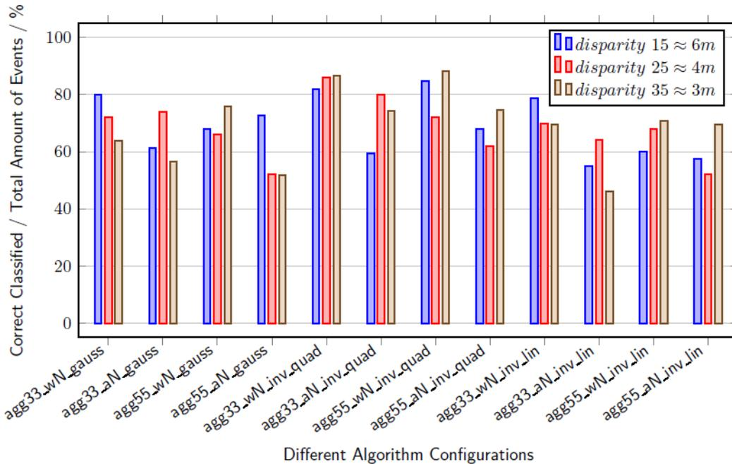
Figure 8. Experimental results of the event-based stereo matching algorithm with different evaluation and algorithm settings.
