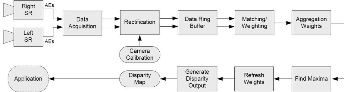
Figure 5. Workflow of the event-based time correlation stereo matching algorithm.
