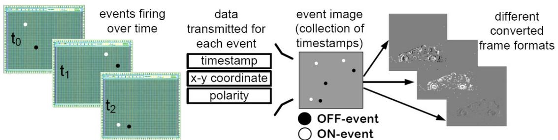
Figure 4. Workflow of the address event to frame converter.
