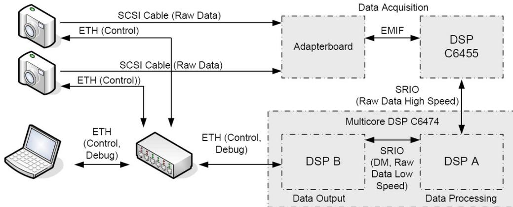
Figure 3. Embedded hardware platform for the data acquisition and execution of the address events from the silicon stereo vision system.
