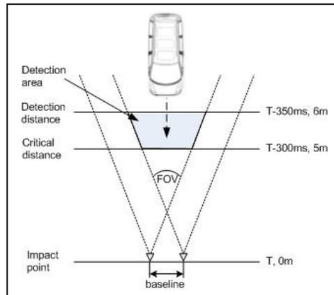
Fig. 3. Overview about the stereo vision system configuration
