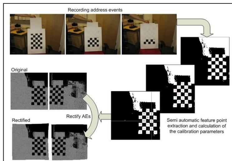
Fig. 4. Calibration and rectification of silicon retina cameras
