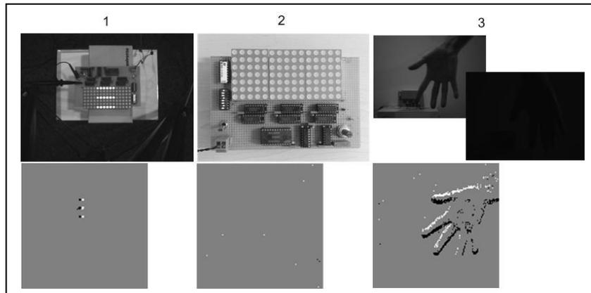
Fig. 2. Advantages of the silicon retina sensor technology, (1) high temporal resolution, (2) data transmission efficiency, (3) wide dynamic range
