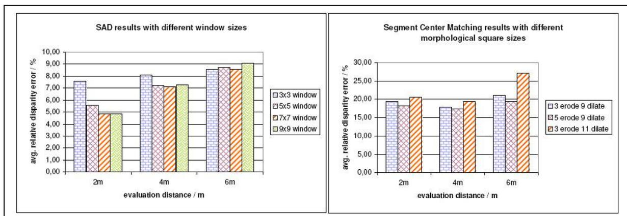
Fig. 5. Results of an area-based (SAD) (left) and of a feature-based (Centre-of-Gravity) (right) algorithm with calibrated and rectified camera data
