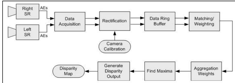
Fig. 6. Blockdiagram of the novel stereo algorithm approach for silicon retina cameras
