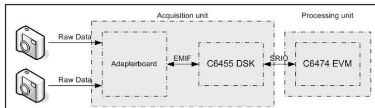
Fig. 7. Overview about the embedded system architecture
