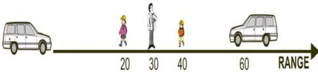
Figure 3. Targets used in simulation. The children at 20 and 40 meters are wearing passive tags.
