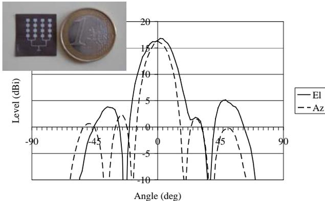
Figure 6. Measured elevation and azimuth cuts of the radiation pattern of fixed-beam high-gain tag antenna.
