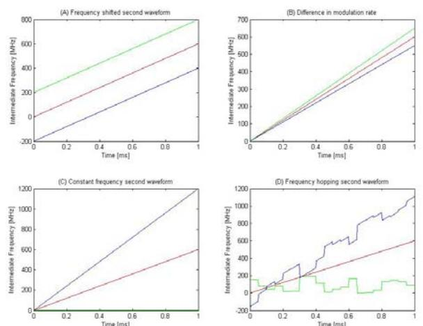
Figure 2. Different harmonic waveforms (in the intermediate frequency band). Base signal 1 and 2 are in red and green respectively. The transponder return signal is in blue.
