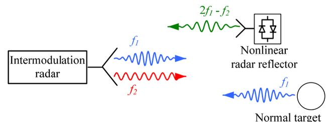
Figure 1. The overall concept of harmonic radar and transponders
