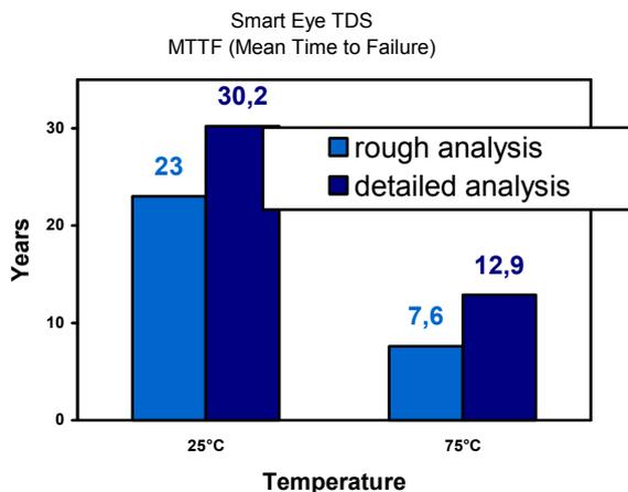
Figure 4. Calculated MTTF for the Smart Eye Sensor
