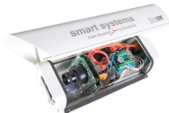
Figure 1. Smart Eye Traffic Data Sensor with opened housing
