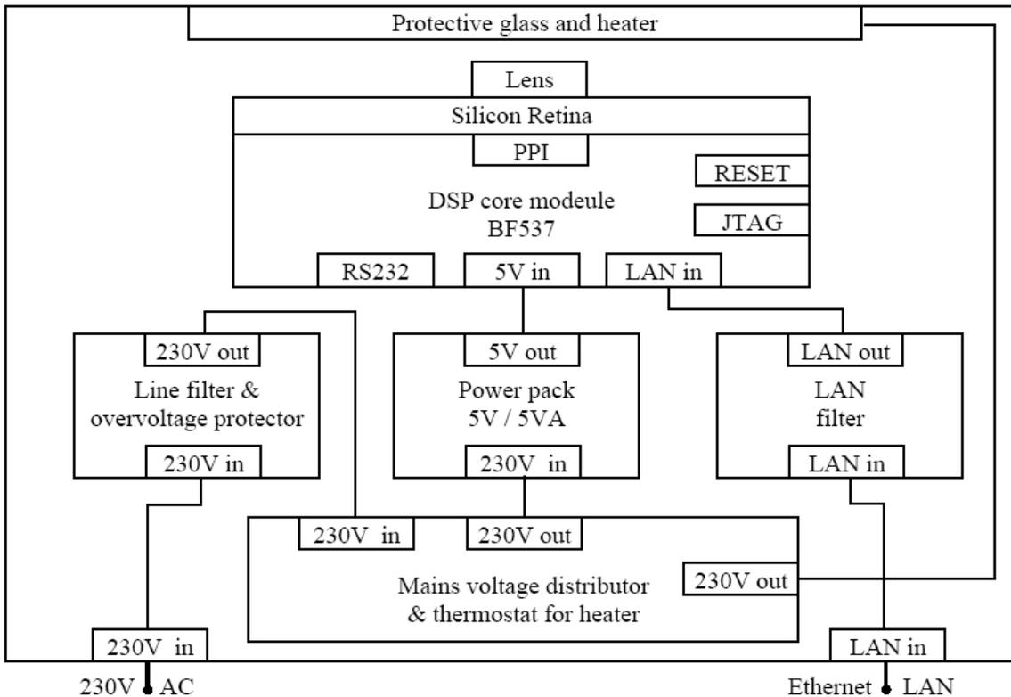
Figure 3. Block diagram of the Smart Eye Sensor
