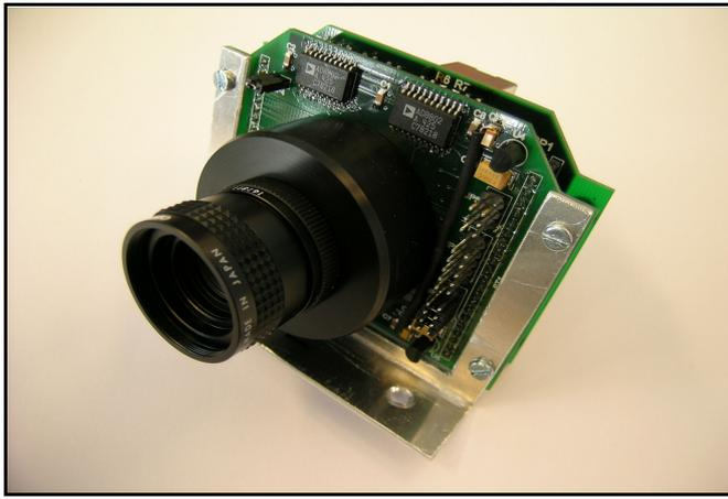
Figure 2. Silicon retina module including lens, optical sensor board and DSP board
