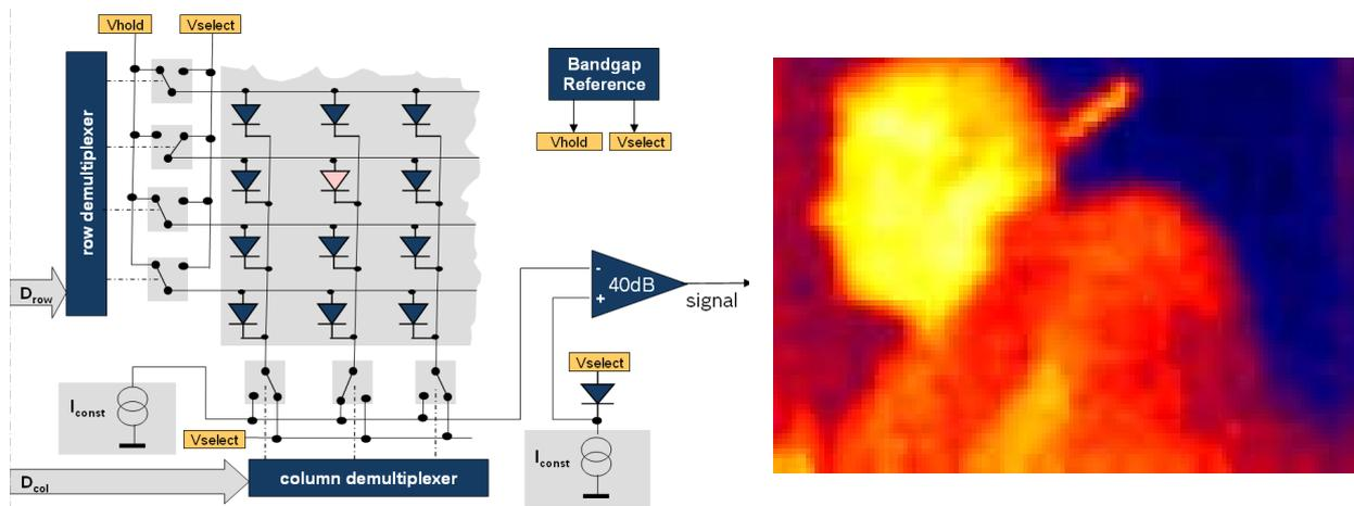
Fig. 8. Basic integrated readout circuit with diode serial addressing for testing (left) and picture taken from a person with the chip (right).
