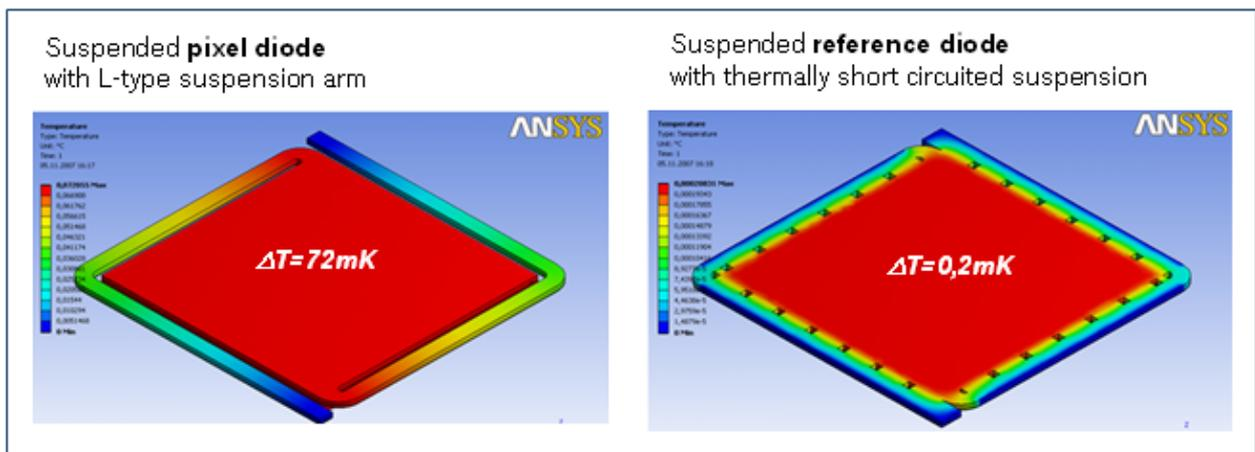
Fig. 5. Pixel diode and reference diode with simulation of the temperature increase from an incident radiant power of 50nW.
