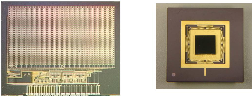
Fig. 6. Photo of the 42 x28 FIR diode test array made with the new process and final vacuum wafer-level packaged chip bonded into a test package.
