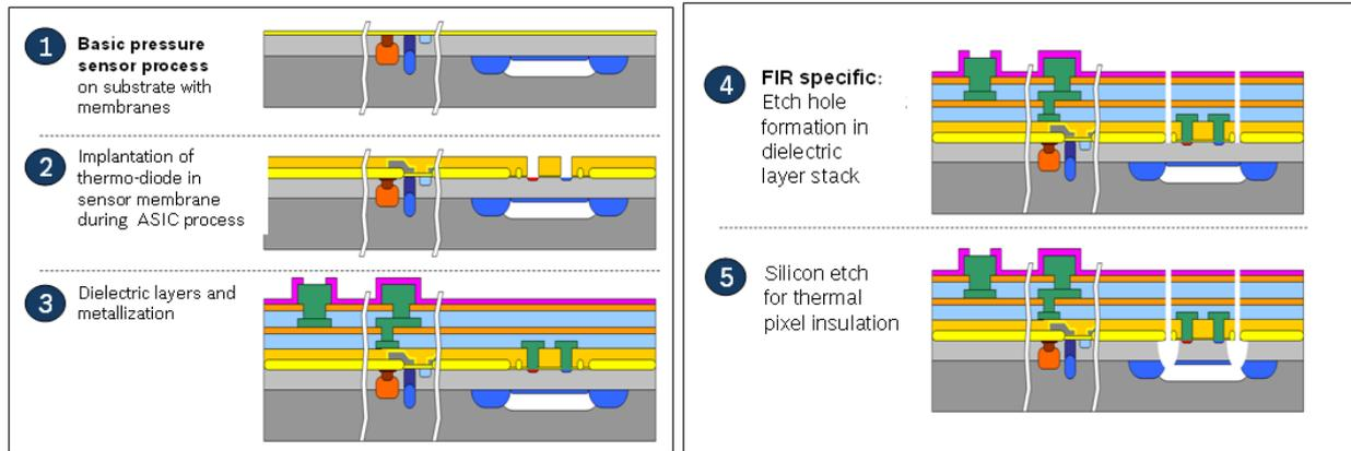
Fig. 4. Basic process flow for the FIR sensor: Steps 1, 2 and 3 schematically represent the steps adapted from the integrated pressure sensor; 4 and 5 show the cavity opening as FIR-array specific process step.
