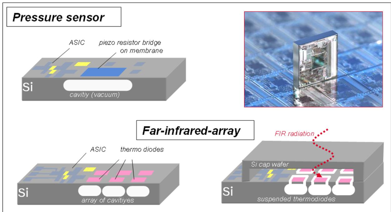
Fig. 3. A production proven integrated MEMS process for surface micro-machined pressure sensors (top) is adapted for manufacturing suspended thermo-diodes for FIR sensor arrays with a single additional mask step and wafer-level vacuum packaging (bottom).
