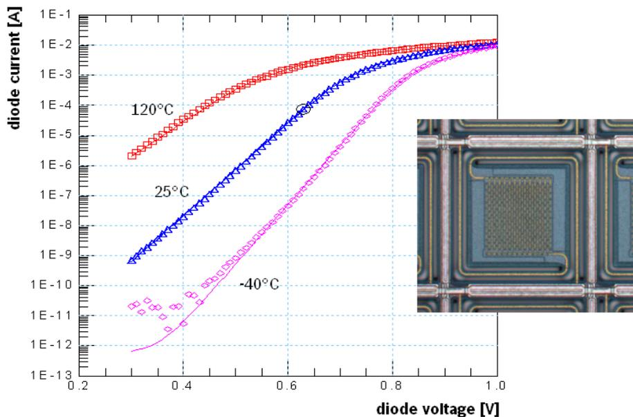
Fig. 7. Current/voltage diagram of a FIR-Diode at different temperatures (left; points: measurement; lines: diode model); photo of a pixel with a suspended thermo-diode (right)
