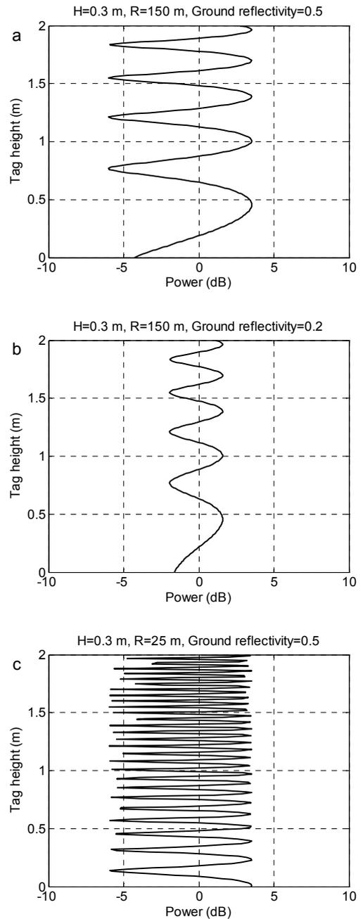
Fig. 2. Variations in received power at the tag as a result of ground reflex.  $H$  is the height above ground of the car radar antenna,  $h$  is the tag height, and  $R$  is the distance between car and tag.
