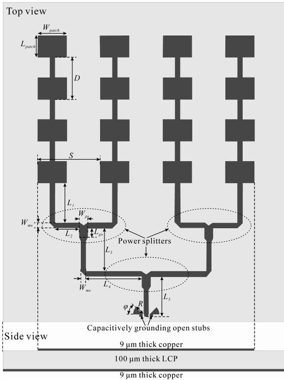
Fig. 3. Layout of the presented tag antenna. Dimensions are:  $L_{patch}=1.04$  mm,  $W_{patch}=1.40$  mm,  $D=2.00$  mm,  $S=3.00$  mm,  $L_1=2.00$  mm,  $L_2=1.12$  mm,  $L_3=2.18$  mm,  $L_4=2.69$  mm,  $L_5=1.81$  mm,  $L_{ps}=480$   $\mu$ m,  $W_{ps}=395$   $\mu$ m,  $W_{ms}=234$   $\mu$ m,  $R=460$   $\mu$ m, and  $\phi=45^\circ$ .
