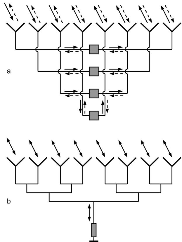
Fig. 1. Comparison between the principle operations of (a) Van Atta array with several transmission-type nonlinear loads and (b) standard array antenna with a single reflective nonlinear load. The Van Atta array gives broader coverage but divides the received power between several loads.
