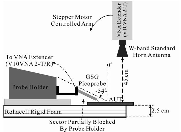
Fig. 5. Measurement setup of antenna radiation properties.
