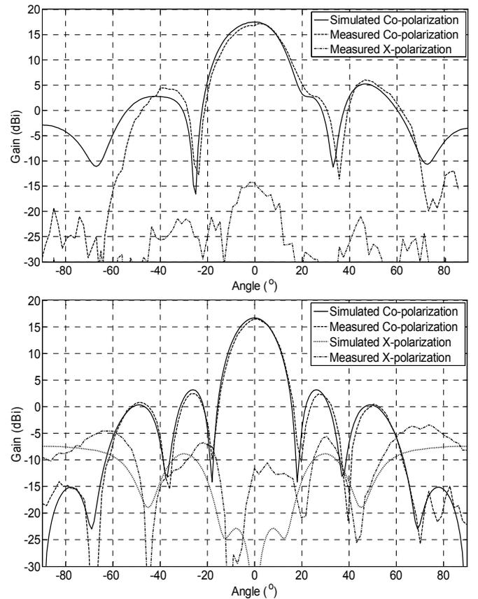
Fig. 6. Simulated and measured radiation patterns, in the vertical plane (upper) and horizontal plane (lower).
