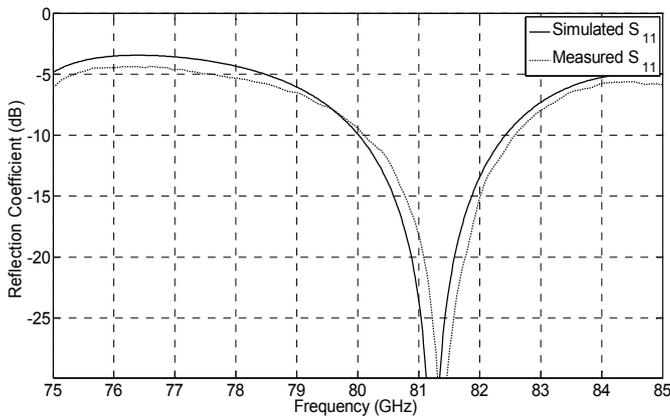
Fig. 4. Simulated and measured reflection coefficients of the array antenna.
