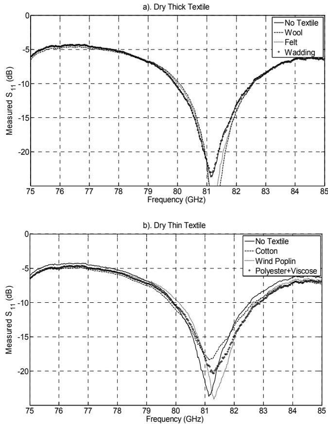
Fig. 7. Measured reflection coefficients of the presented tag antenna with various dry textile layers in front of it.
