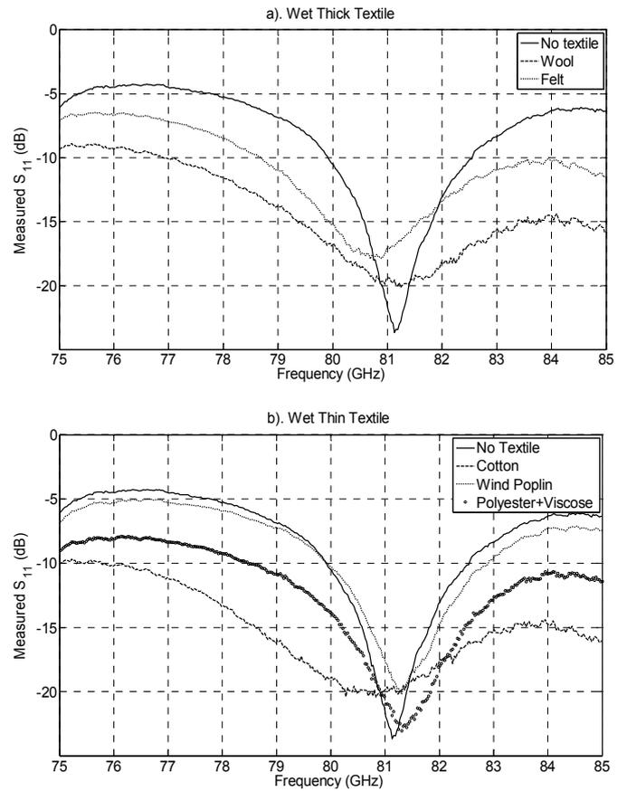
Fig. 8. Measured reflection coefficients of the presented tag antenna with various textile layers in front of it, all soaking wet.
