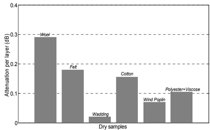
Fig. 8. Attenuation (gain reduction) due to of various dry textile layers in front of the antenna.
