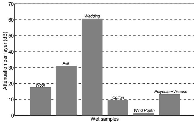
Fig. 9. Attenuation (gain reduction) due to of various textile layers in front of the antenna, all soaking wet.
