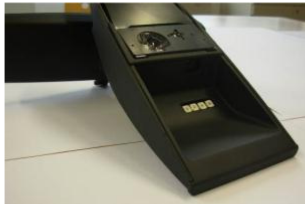
Figure 2 - MFOS camera prototype integrated in the internal rearview mirror
