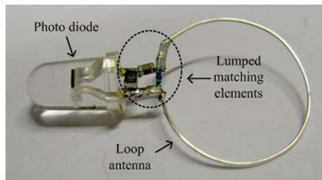
**Figure 3** A photograph of the photo-activated microwave transponder. [Color figure can be viewed in the online issue, which is available at [www.interscience.wiley.com](http://www.interscience.wiley.com)]
