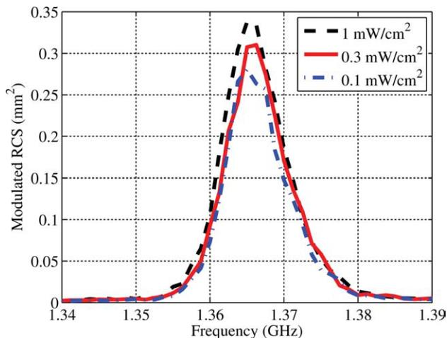
**Figure 4** The measured modulated radar cross section (RCS) of the transponder. The curves are for different irradiance levels. [Color figure can be viewed in the online issue, which is available at [www.interscience.wiley.com](http://www.interscience.wiley.com)]
