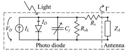
**Figure 1** An electrical equivalent circuit of the wireless photo detector
