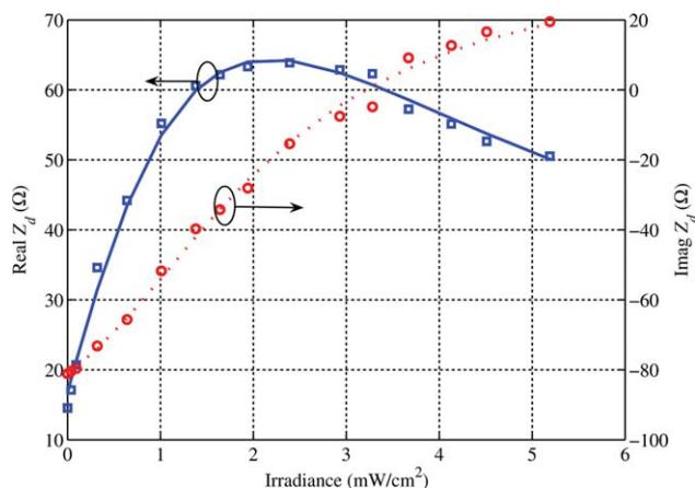
**Figure 2** The measured (marker) and calculated (line) impedance of the photo diode at 1.5 GHz as a function of irradiance. [Color figure can be viewed in the online issue, which is available at [www.interscience.wiley.com](http://www.interscience.wiley.com)]
