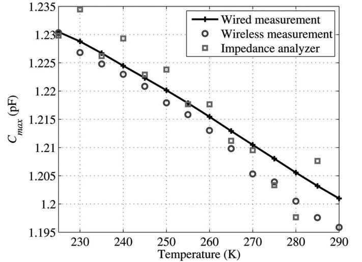
Fig. 6. The measured temperature responses of the sensor.
