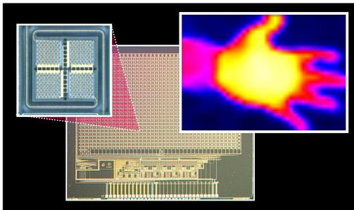
Technology test chip and FIR-image accessed
