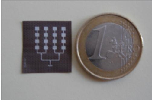
Four-by-four element wearable array antenna.
