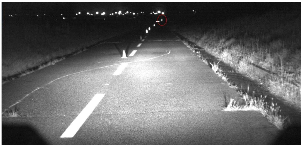
Figure 4: Low beams and IR illuminators. Pedestrian at 100m
