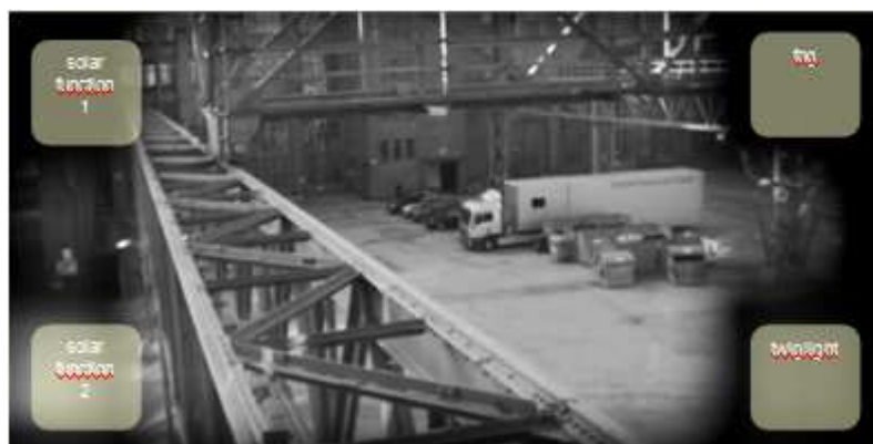
Figure 7: Functional indication of the ROI in the 4 corners of the chip image. The markers are transparent. The solar function in the left down corner is more bright indicating sun light coming from the left side
