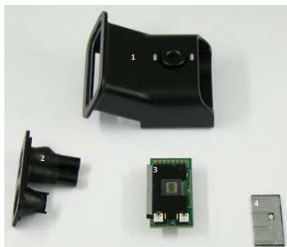
Figure 3: Prototype component parts: 1) housing with imager optic; 2) LED mirror and fog/twilight optic; 3) imager chip with mounting for the lightpipes; 4) lightpipes coated with aluminium
