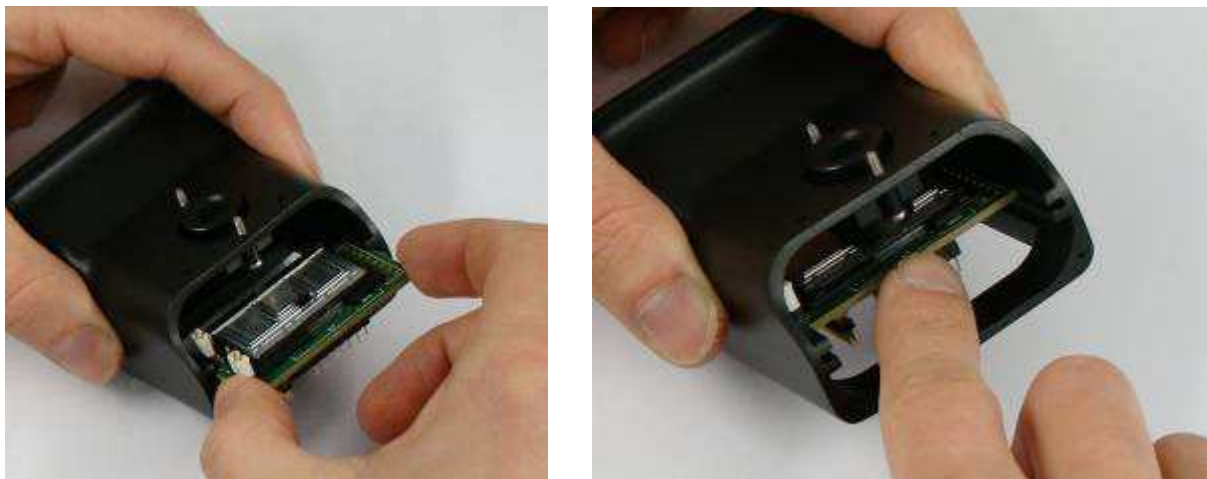
Figure 5: Step 2 - push the electronic in to the housing
