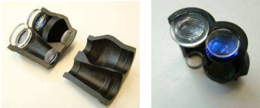
Figure 2: Lens holder made by rapid prototyping with lenses and IR-filter
